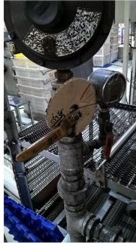
Figure IV.4: The roasting gas flow rate lever with cardboard dial marked with levels used in experiments
