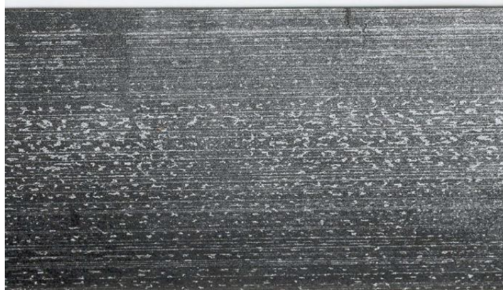
Figure 2-7: Typical pitting corrosion.
