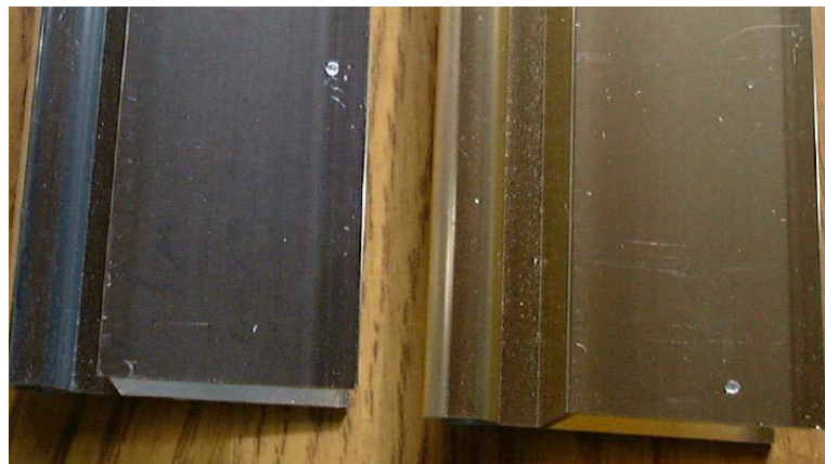
Figure 2-9: Structural of die design streaking
