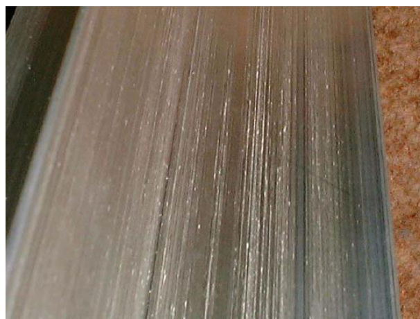
Figure 2-8: Die line defect on the extruded aluminum.
