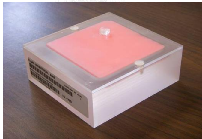
Figure3. 5 Mammography phantom image Quality Evaluation: ACR breast phantom model RMI 156.
