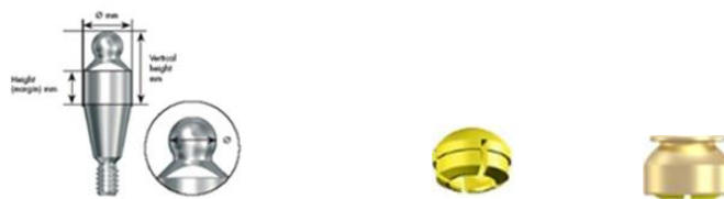
Figure 8 Schematic diagram of structure of ball attachments; height of ball attachment - 2.00 mm, diameter of ball attachment - 2.25 mm.
