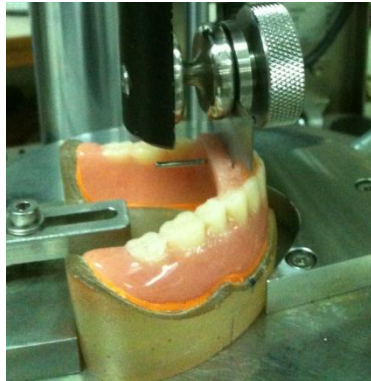
Figure 7 A stainless steel plate connected the overdenture to the universal testing machine
