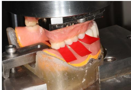
Figure 6 All upper teeth were in contact when checked with shim stock
