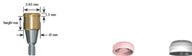
Figure 9 Schematic diagram of structure of Locator attachments; height of Locator attachment - 2.00 mm, diameter of Locator attachment - 3.85 mm.
