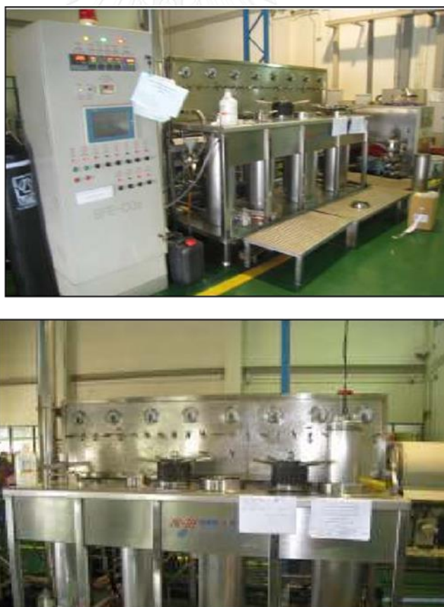
Figure 9. Supercritical fluid extraction apparatus (Model: 24L-SFE, China).
