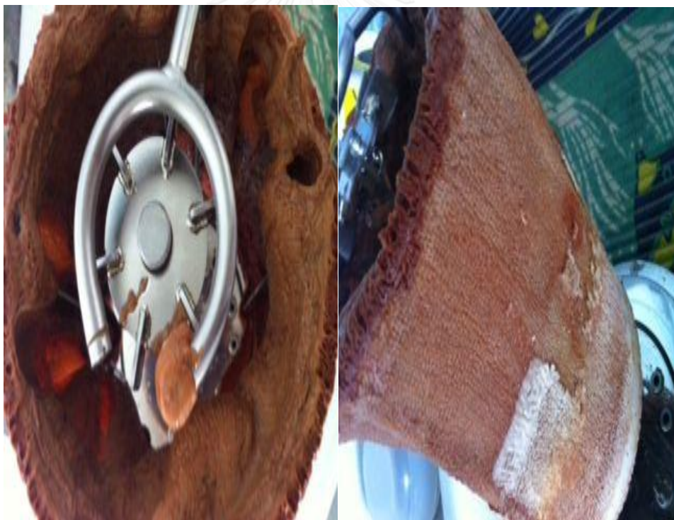
Figure 4. 4 Morphology of A.terreus immobilized on the cotton cloth in the static bed bioreactor at 30 °C and pH2 for 7 days.
