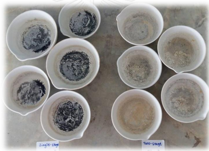
Figure 4.23 Single-stage and two-stage digestate after burning in furnace at 550°C for 20 minutes
