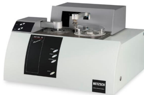
Figure 3.4 Differential scanning calorimetry (DSC) [47]
