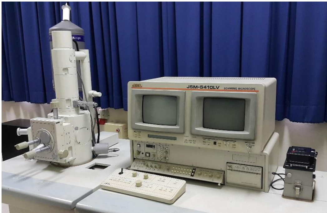
Figure 22: Scanning electron microscope (JSM-5410LV, JEOL, Japan) and energy dispersive x-ray microanalysis (Model 6647, Oxford Instruments, England)
