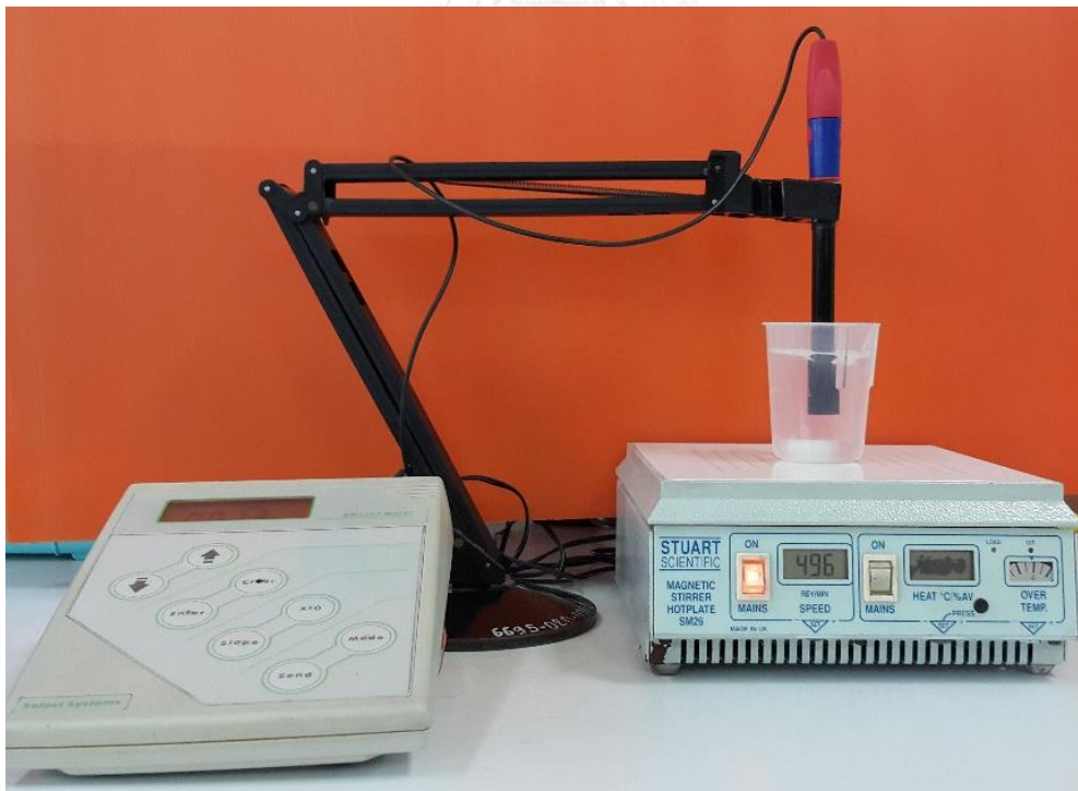
Figure 21: Fluoride ion-selective electrode (Model SL518, Select Bioscience, English) and expandable ion analyzer (QI518C, Q-I-S, Netherlands)
