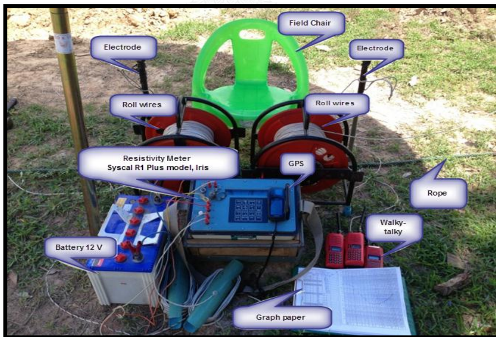
Figure 4.5 Equipment of the VES survey.
