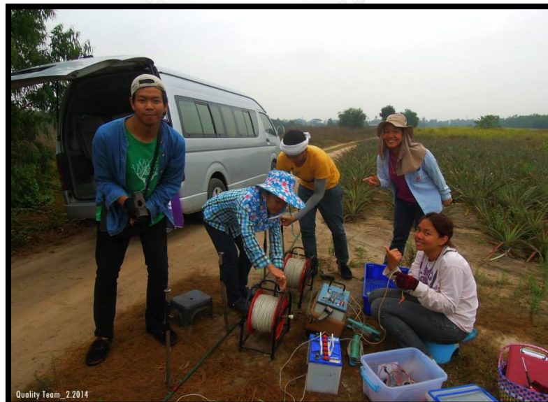
Figure 4.7 Resistivity Meter showing channels connected to points A, B, M and N.
