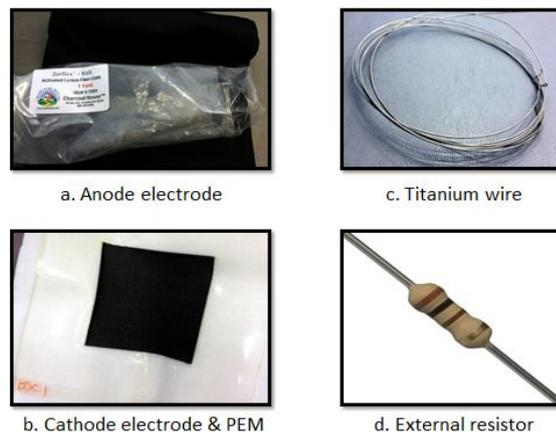
**Figure 3.6** Electrical equipment in MFCs a) anode electrode, b) cathode electrode and PEM, c) titanium wire, and d) external resistance
