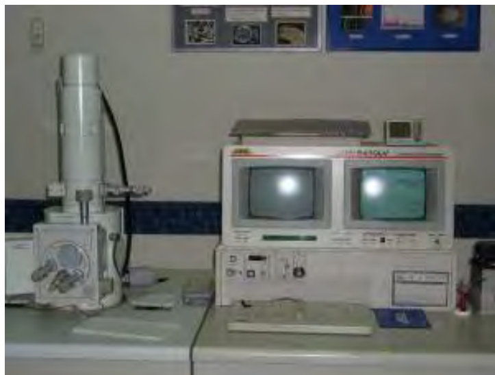
Figure 3.2 Scanning electron microscope (SEM) (Jeol model JSM-6400)
