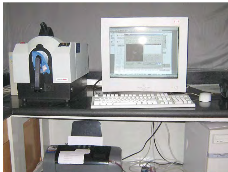
Figure 3.5 Computer color matching machine (CCM) (Macbeth color eye 3100)
