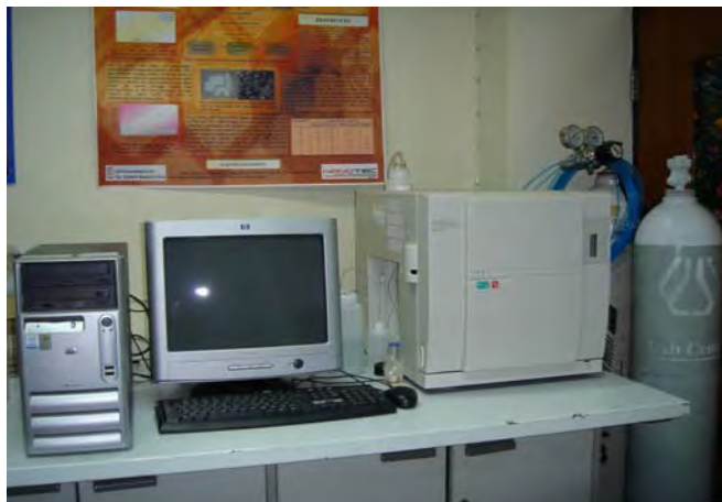
Figure 3.7 Total organic carbon analyzer (TOC) (Shimadzu TOC-VCPH)
