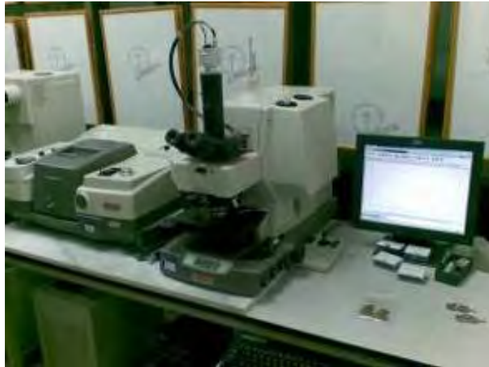
Figure 3.3 Fourier transform infrared spectrometer (FT-IR) (model1760x)
