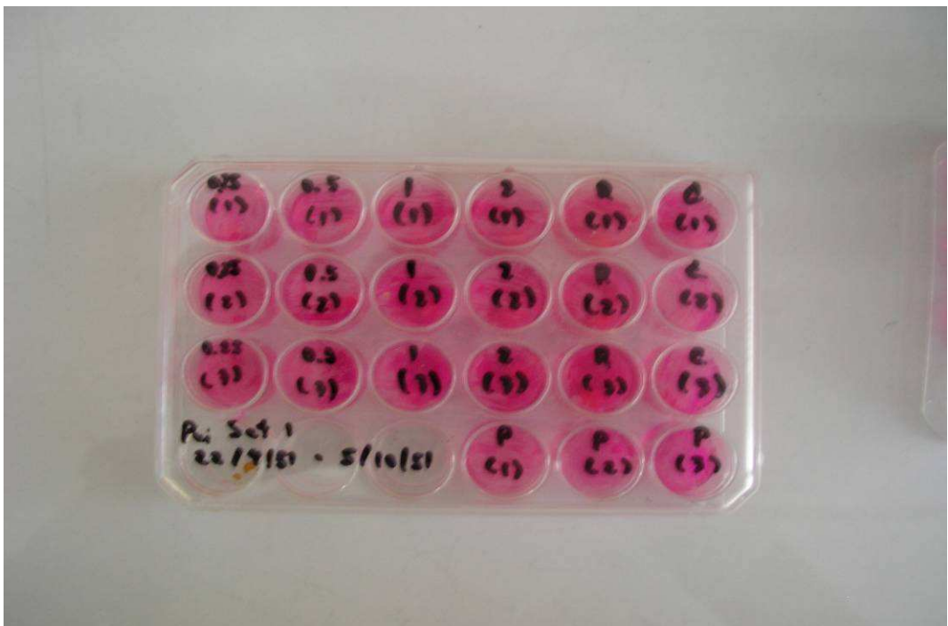
A 32. Immersion of materials into fibroblast media for 24, 48 and 72 hrs.
