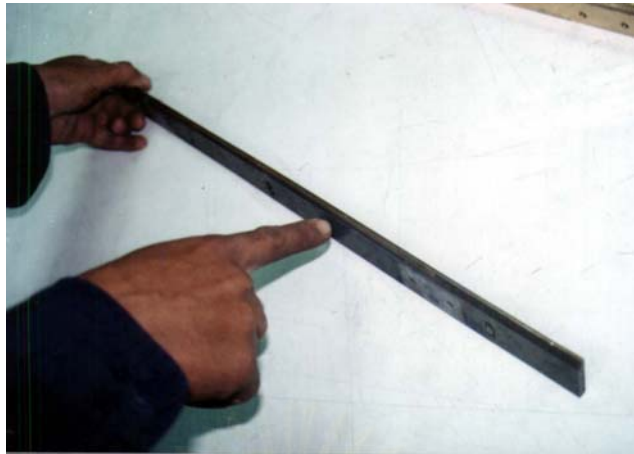
Figure 5.7 The Thickness Adjustment Plate was worn
