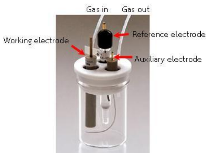
Figure 2.4 An electrochemical cell
