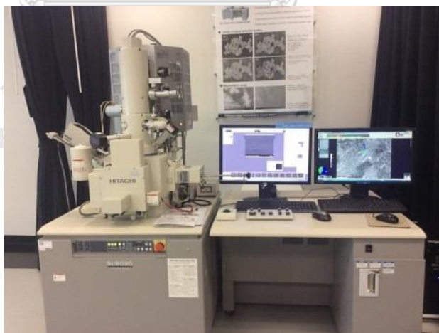
Figure 4.4: Energy dispersive x-ray spectroscopy detector used in conjunction with Field emission scanning electron microscope (HITACHI SU8030).
