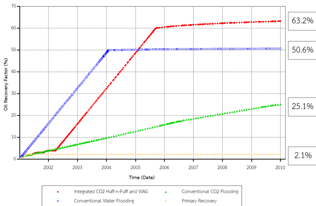
Figure 4.26 Comparison of oil recovery factor between integrated CO 2 Huff-n-Puff and WAG and other oil recovery processes
