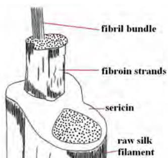
Figure 2.1 Structure of silk fiber [12]
