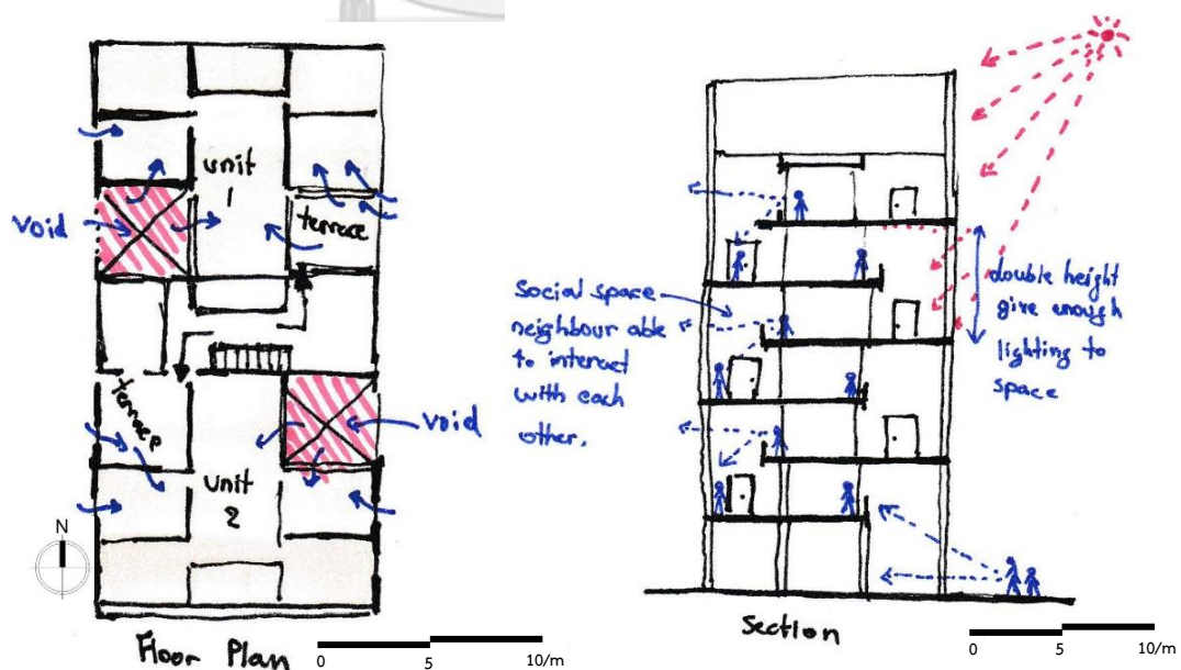
Figure 2. 65 Diagram drawing analysis of the unit floor plan and section of the building
