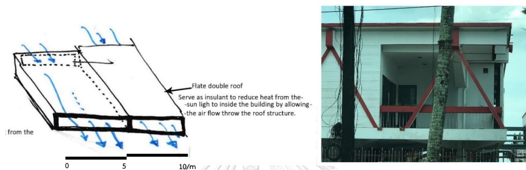
Figure 2. 8 Flat double roof design with the two-layer structure that serves as an insulation, reducing the heat caused due to the sunlight
