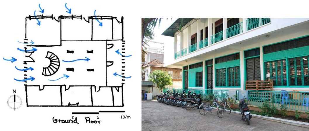
Figure 2. 60 Drawing analysis of air circulation on the ground floor, the cantilevers of the upper floor, which provide shade to the glass curtain below
