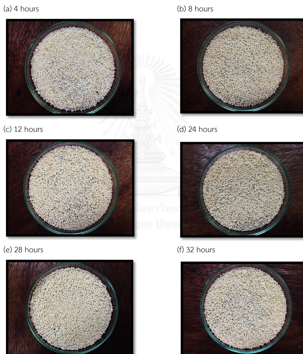
Figure 4.43 25%GLU-2%CHI-15%STY/PS beads obtained at 80°C for (a) 4 hours (b) 8 hours (c) 12 hours (d) 24 hours (e) 28 hours and (f) 32 hours of glutaraldehyde-treated time
