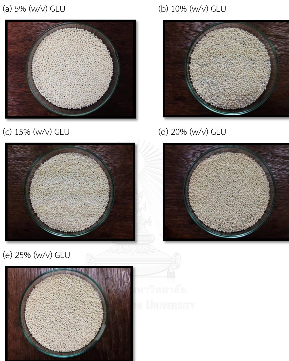
Figure 4.36 Comparison of 3%CHI-15%STY/PS beads activated with various concentrations of glutaraldehyde solution at 80°C for 24 hours (a) 5% (w/v) GLU (b) 10% (w/v) GLU (c) 15% (w/v) GLU (d) 20% (w/v) GLU and (e) 25% (w/v) GLU
