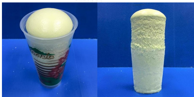
Figure 4.5 RPUR foams prepared by using a 700 ml plastic cup and catalyzed by \text{Cu}(\text{OAc})_2(\text{en})_2/\text{Sal} at the mole ratio of 1:1
