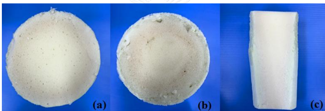
Figure 4.43 RPUR foams catalyzed by \text{Cu}(\text{OAc})_2(\text{en})_2/\text{Ac} (1:2) (a) top; (b) bottom; (c) side of the foam sample
