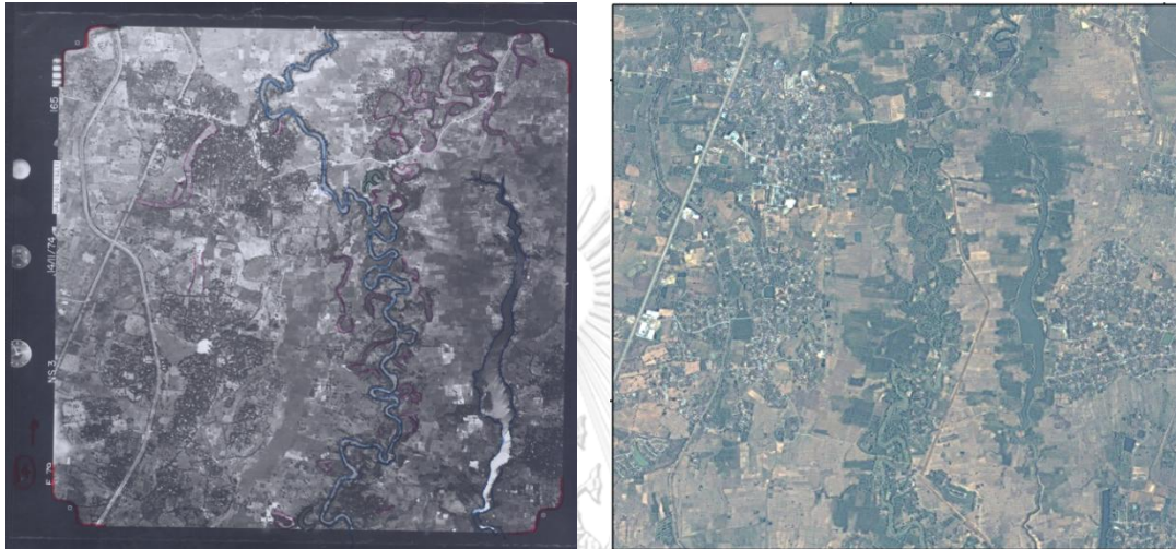
Figure 20 The printed versions of historical aerial photographs in 1974 scale 1:15,000 (left) and satellite image from THEOS1 Satellite image in 2011 (right) were used to examine the geomorphological change of the Mun River in Amphoe Khon Buri and Chok Chai.
