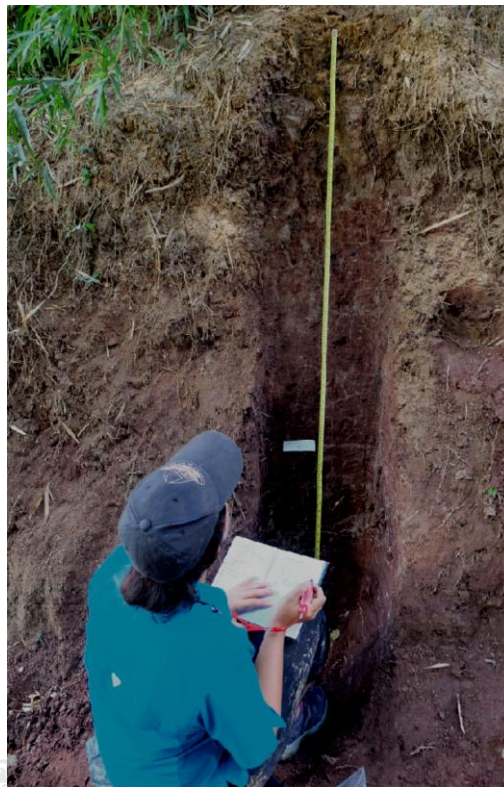
Figure 28 The bank site was trenched to get fresh exposures, and the detailed descriptions of the stratigraphy were made at each site including the size, color, and texture.
