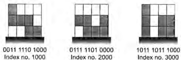
Figure 2 Examples of chromosome encoding and index. Shaded areas indicate filled grids while white grids are empty.
