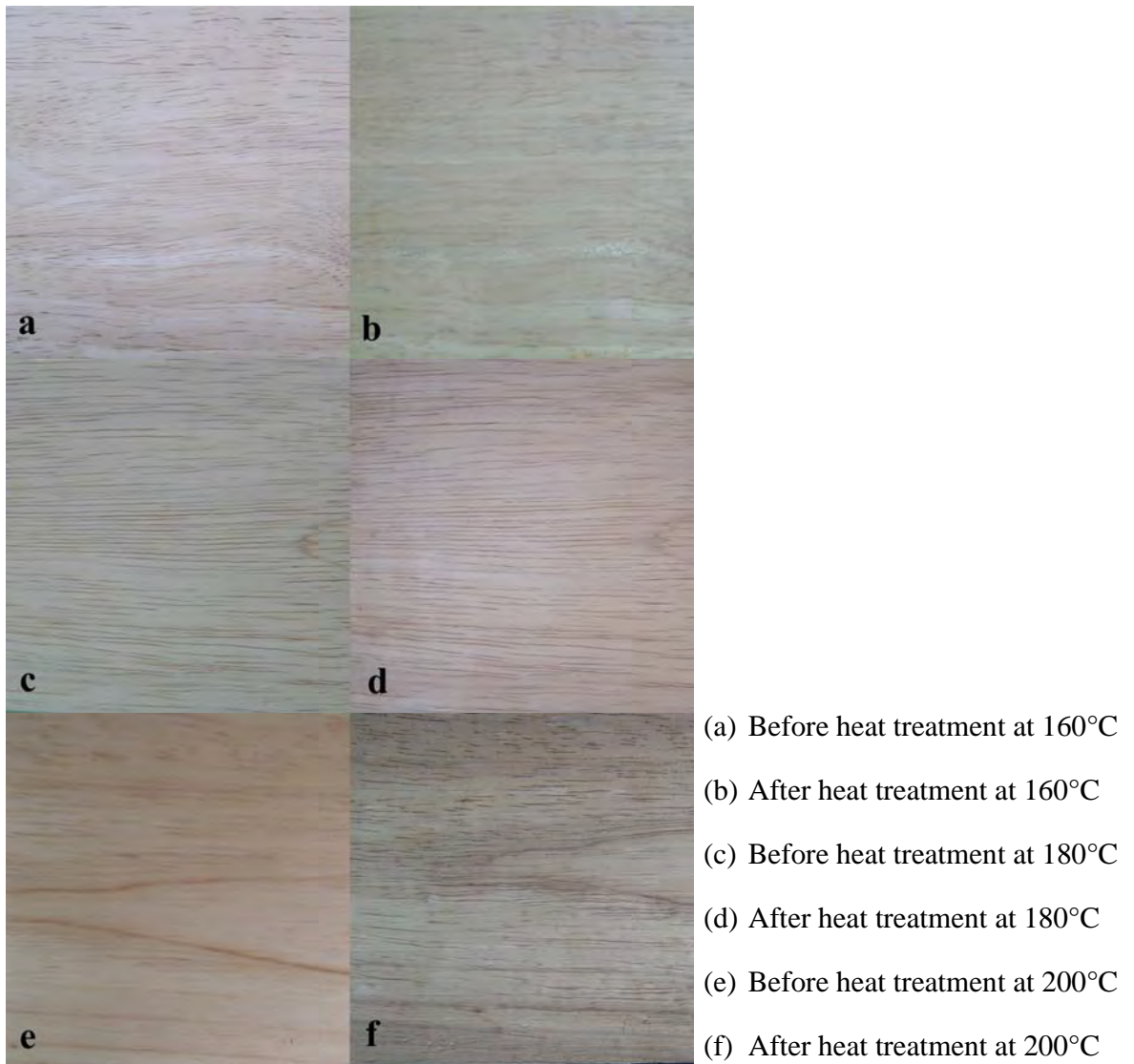
Figure 4.12 Comparison of rubberwood before and after heat treatment at 160-200°C
