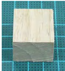
Figure 3.2 Dimension of testing samples for water contact angle and decay test.
