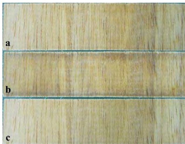
Figure 4.25 Comparison of water absorption test of treated rubberwood with 12% loading of ETO (a) before test (b) after test (c) after test 24 h.
