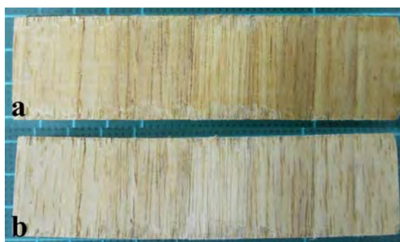
Figure 4.28 Comparison of water absorption test of treated rubberwood with methyl ester of tung oil (a) before test (b) after test.
