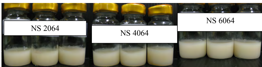
Figure 29 The photograph of niosome serum formulations with 0.5% emblica extract loaded niosomes, under storage condition at room temperature (30 °C) at 12 weeks
