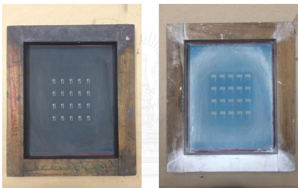
Figure 3.1 Screen-printing blocks for working and counter electrode (left) and silver-silver chloride reference electrode and conducting pads (right).
