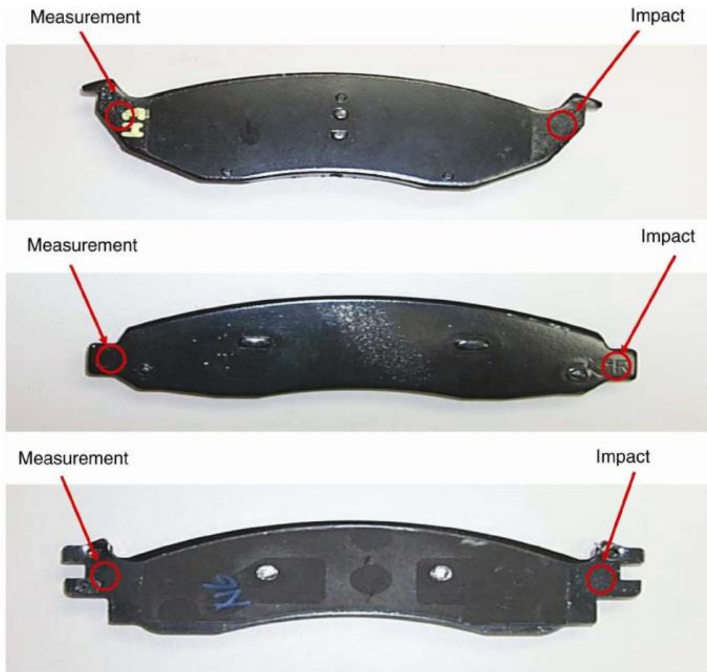
FIGURE 2—BRAKE PAD NATURAL FREQUENCY AND LOSS FACTOR MEASUREMENT CONFIGURATION NUMBER 1
