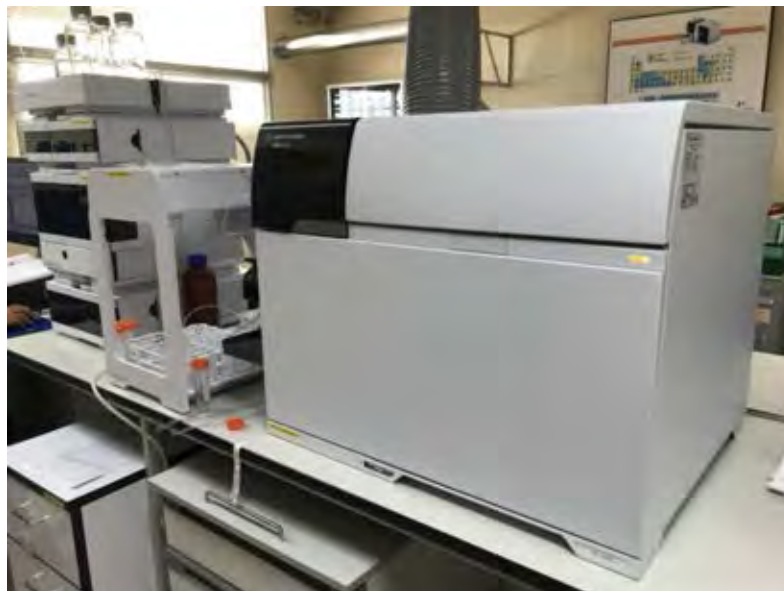
Fig 3.10 Inductively Coupled Plasma Optical Emission Spectrometry (ICP-MS)
