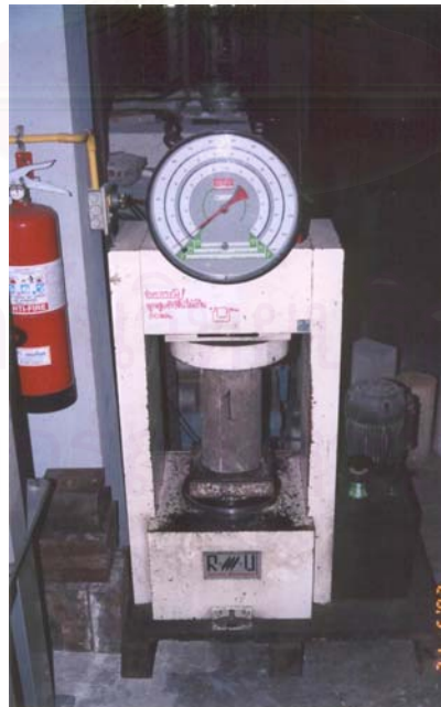
Figure B-4 Compressive Strength Testing Machine
