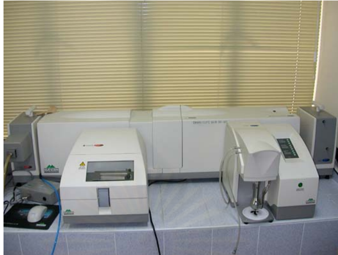
Figure B-7 The Particle Size Analyzer Model Mastersizer 2000 and Scirocco 2000
