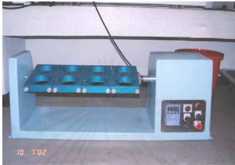
Figure B-1 The Rotary Agitator
