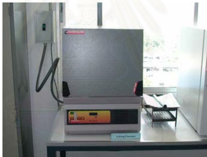
Figure B-6 The Ashing Furnace Model AAF 1100
