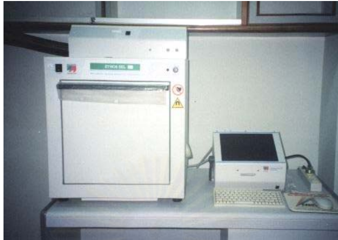
Figure B-5 The Microwave Digestion and Extraction Apparatus Model ETHOS SEL
