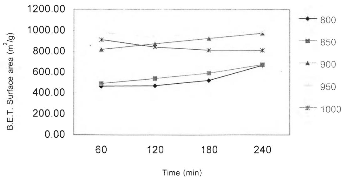
Figure 4.18 Effect of time on B.E.T. surface area at different time (size 1.18 – 2.36 mm, 10 g, air 0.005 l/min, CO<sub>2</sub> 0.5 l/min and H<sub>2</sub>O 0.01 l/min).
