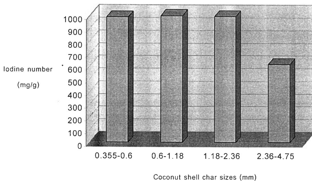
Figure 4.20 Effect of size on iodine number (air 0.005 l/min, CO<sub>2</sub> 0.5 l/min and superheated steam at the flow rate of 10 g/min, 10g, 60 min, 950<sup>o</sup>C).
