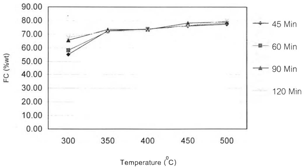
Figure 4.6 Effect of temperature on % fixed carbon at different times.
