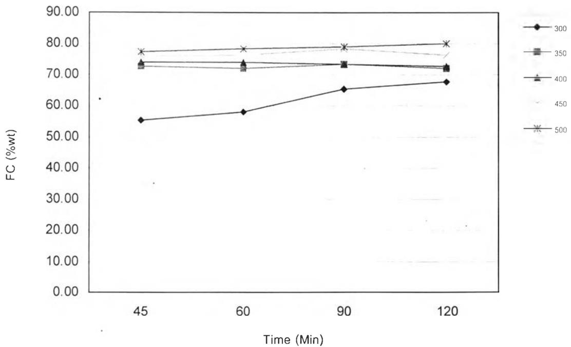
Figure 4.10 Effect of time on % fixed carbon at different times.
