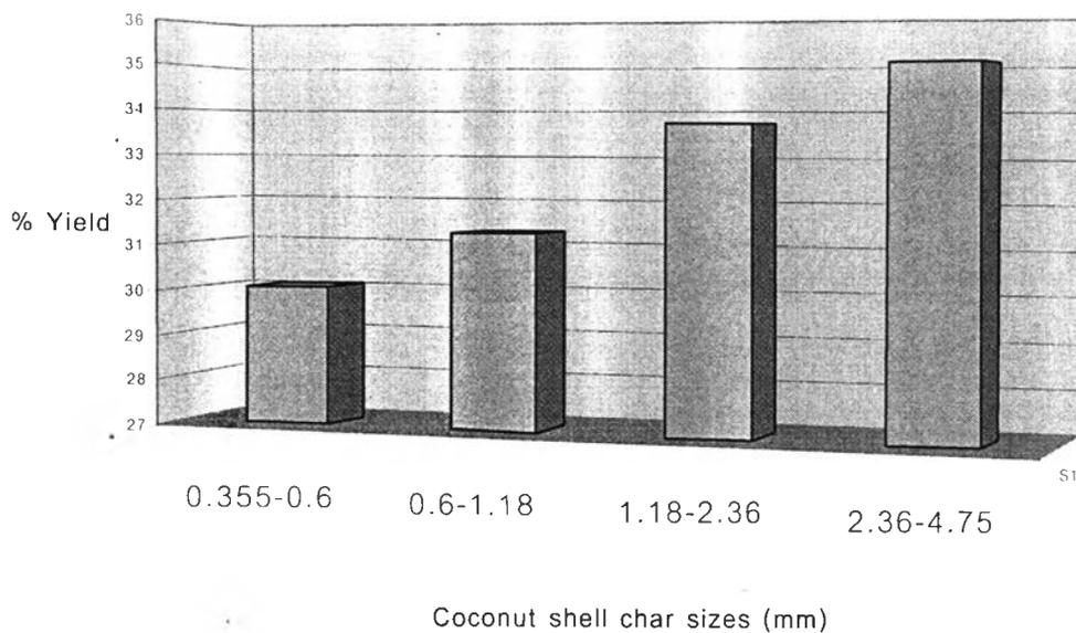
Figure 4.19 Effect of size on % yield (air 0.005 l/min, CO<sub>2</sub> 0.5 l/min and superheated steam at the flow rate of 10 g/min, 10g, 60 min, 950<sup>o</sup>C).
