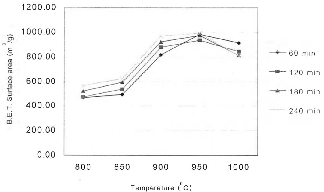
Figure 4.14 Effect of temperature on B.E.T. surface area at different time (size 1.18 – 2.36 mm, 10 g, air 0.005 l/min, CO<sub>2</sub> 0.5 l/min and H<sub>2</sub>O 0.01 l/min).
