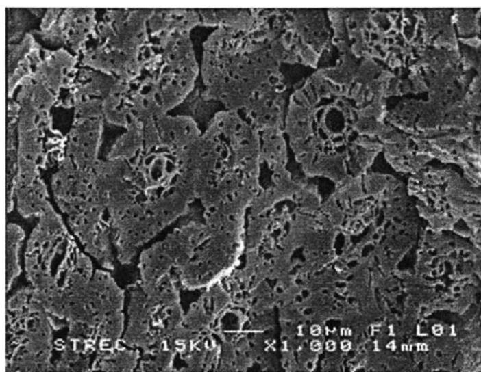
Figure 4.28 Activated carbon from coconut shell sizes 0.6-1.18, 950<sup>o</sup>C 1 hr., flow rate of air 0.005 l/min and flow rate of pure superheated.
