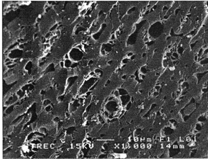
Figure 4.29 Activated carbon from coconut shell sizes 0.6-1.18, 950<sup>0</sup>C 60 min, flow rate of air 0.005 l/min and carbon dioxide at composition 8%
