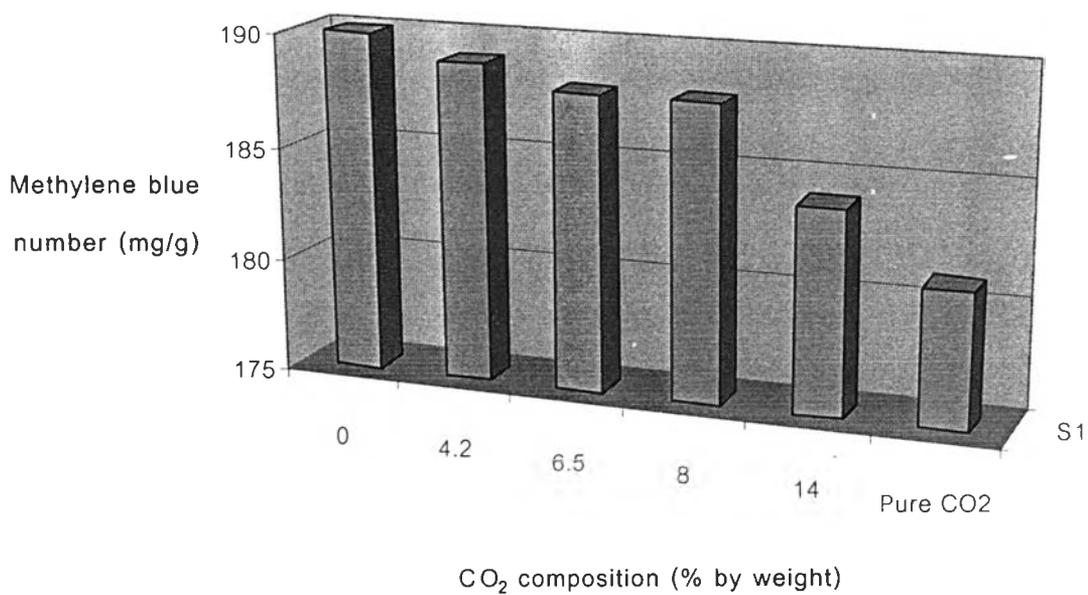
Figure 4.25 Effect of CO<sub>2</sub> (% weight) composition on methylene blue number (950<sup>0</sup>C for 60 min, 0.60-1.18, 10g, air 0.005 l/min and superheated steam 10 g/min).
