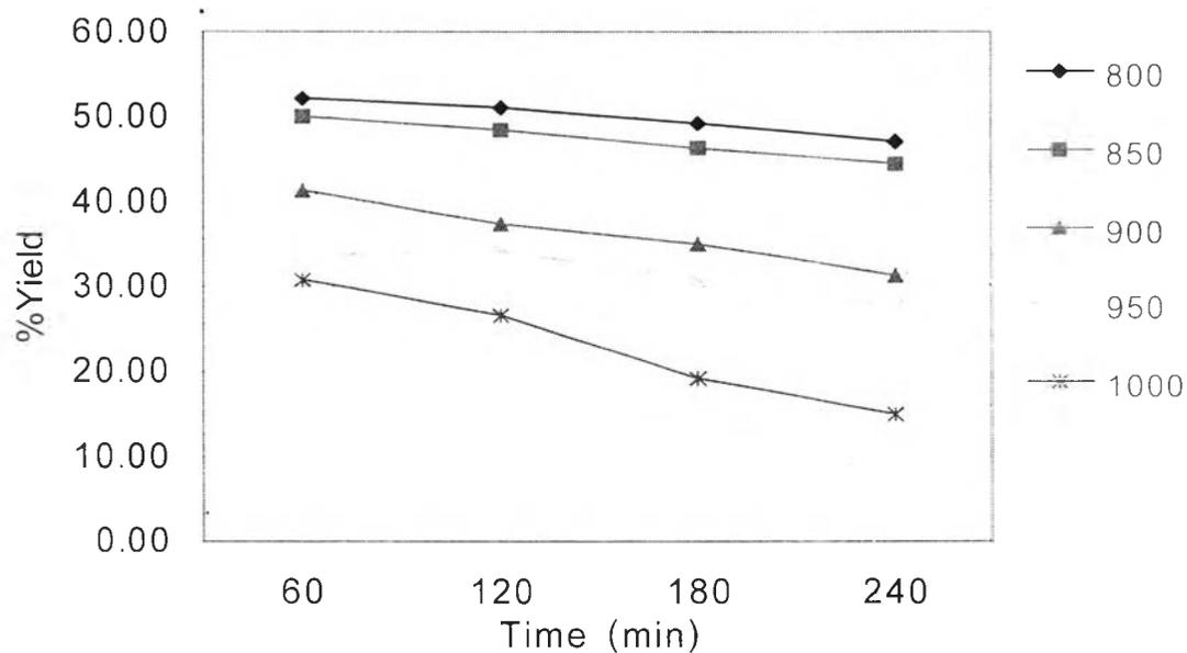
Figure 4.15 Effect of time on % yield at different time (size 1.18 – 2.36 mm, 10 g, air 0.005 l/min, CO<sub>2</sub> 0.5 l/min and H<sub>2</sub>O 0.01 l/min).
