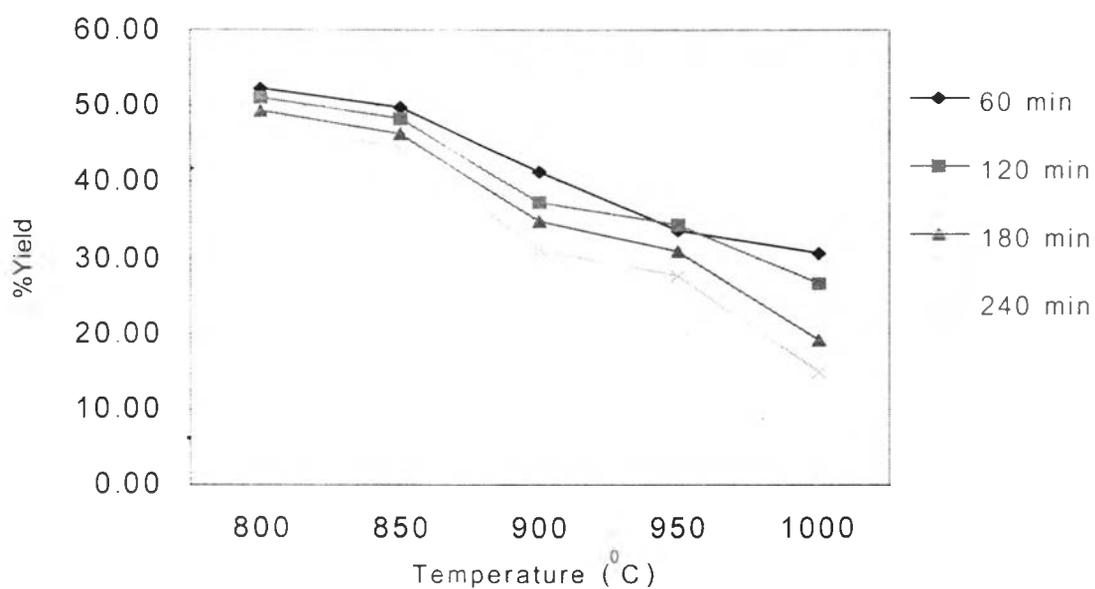
Figure 4.11 Effect of temperature on % yield at different time (size 1.18 – 2.36 mm, 10 g, air 0.005 l/min, CO<sub>2</sub> 0.5 l/min and H<sub>2</sub>O 0.01 l/min).
