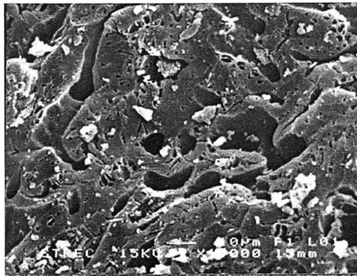
Figure 4.30 Activated carbon from coconut shells sizes 0.6-1.18, 950<sup>0</sup>C 60 min, flow rate of air 0.005 l/min and pure carbon dioxide.
