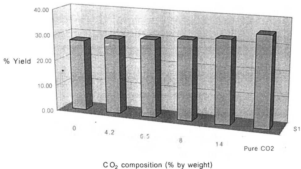
Figure 4.23 Effect of CO<sub>2</sub> (% weight) composition on % yield (950<sup>0</sup>C for 60 min, 0.60-1.18, 10g, air 0.005 l/min and superheated steam 10 g/min).
