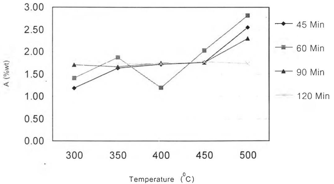
Figure 4.4 Effect of temperature on % ash at different times.
