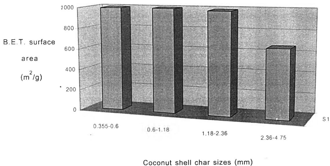
Figure 4.22 Effect of size on B.E.T. surface area (air 0.005 l/min, CO<sub>2</sub> 0.5 l/min and superheated steam at the flow rate of 10 g/min, 10g, 60 min, 950<sup>0</sup>C).
