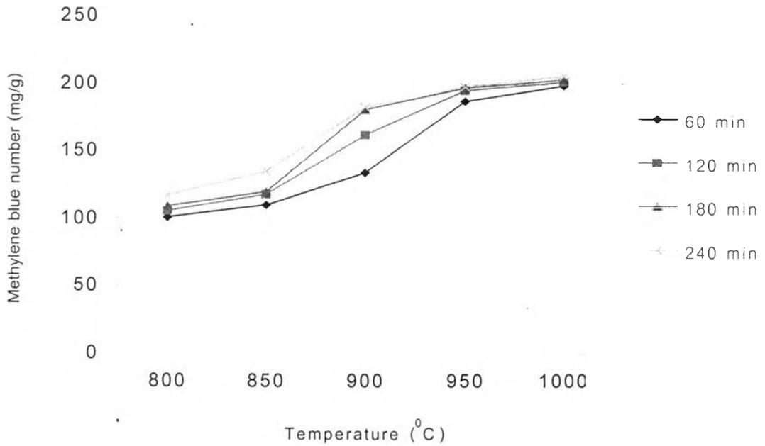
Figure 4.13 Effect of temperature on methylene blue number at different time (size 1.18 – 2.36 mm, 10 g, air 0.005 l/min, CO<sub>2</sub> 0.5 l/min and H<sub>2</sub>O 0.01 l/min).
