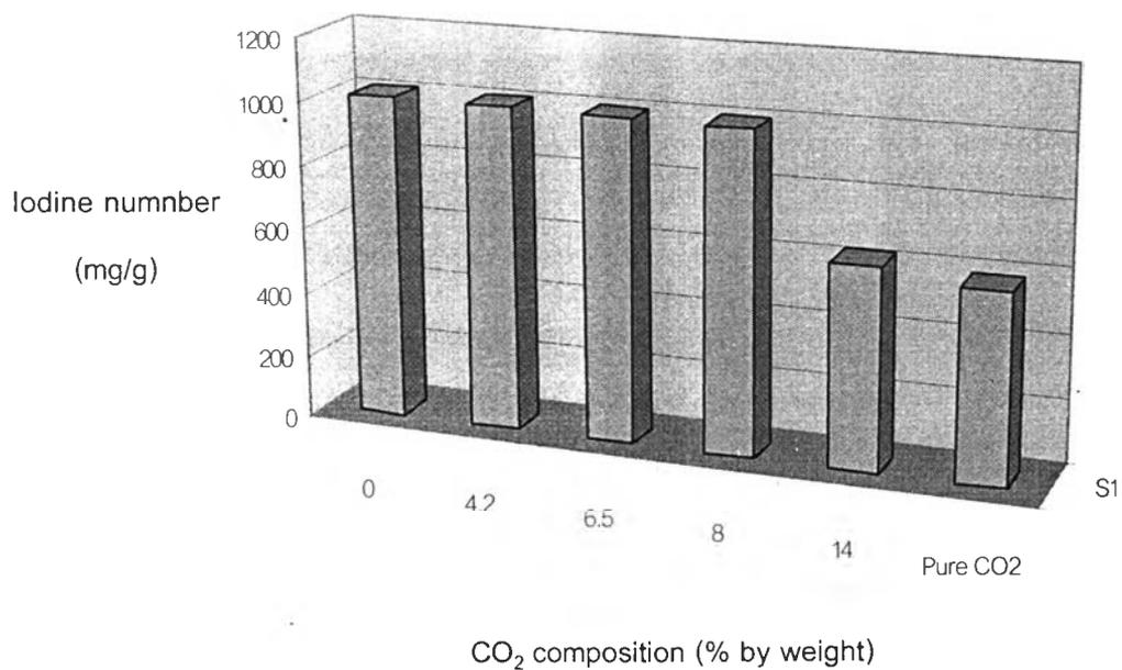
Figure 4.24 Effect of CO<sub>2</sub> (% weight) composition on iodine number (950<sup>0</sup>C for 60 min, 0.60-1.18, 10g, air 0.005 l/min and superheated steam 10 g/min).
