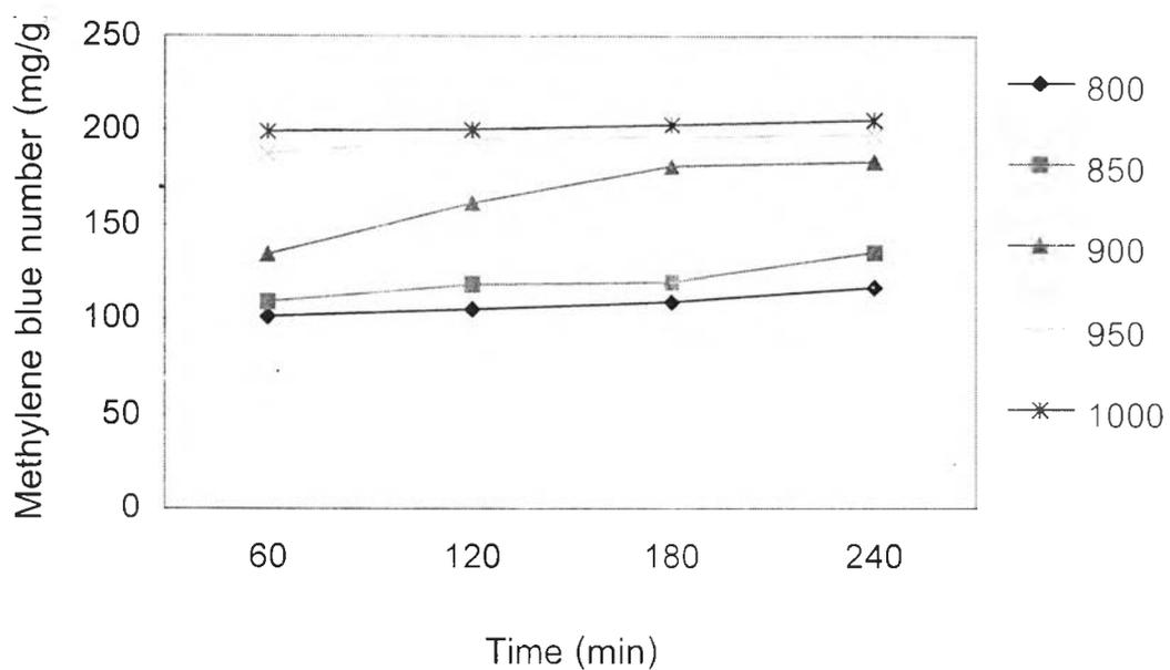
Figure 4.17 Effect of time on methylene blue number at different time (size 1.18 – 2.36 mm, 10 g, air 0.005 l/min, CO<sub>2</sub> 0.5 l/min and H<sub>2</sub>O 0.01 l/min).
