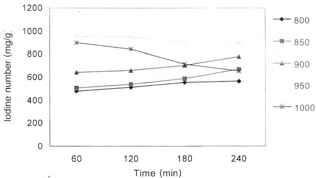
Figure 4.16 Effect of time on iodine number at different time (size 1.18 – 2.36 mm, 10 g, air 0.005 l/min, CO<sub>2</sub> 0.5 l/min and H<sub>2</sub>O 0.01 l/min).
