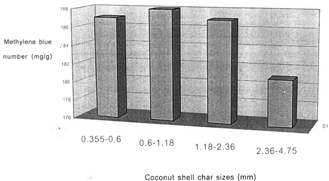
Figure 4.21 Effect of size on methylene blue number (air 0.005 l/min, CO<sub>2</sub> 0.5 l/min and superheated steam at the flow rate of 10 g/min, 10g, 60 min, 950<sup>0</sup>C).
