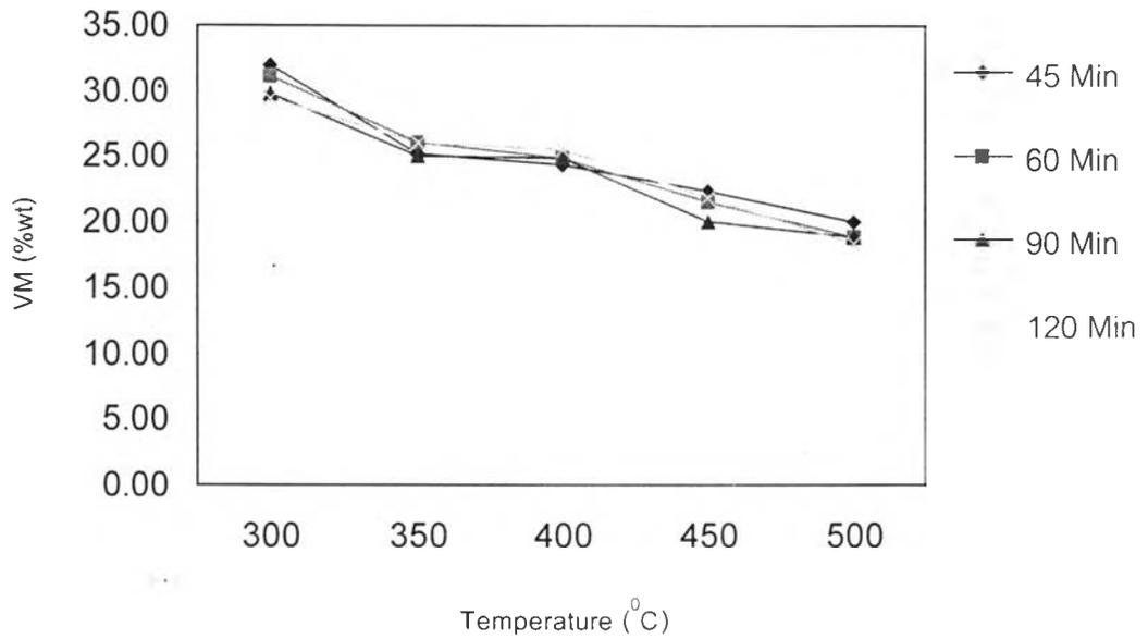
Figure 4.5 Effect of temperature on % volatile at different times.
