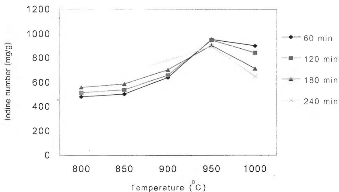
Figure 4.12 Effect of temperature on % iodine number at different time (size 1.18 – 2.36 mm, 10 g, air 0.005 l/min, CO<sub>2</sub> 0.5 l/min and H<sub>2</sub>O 0.01 l/min).
