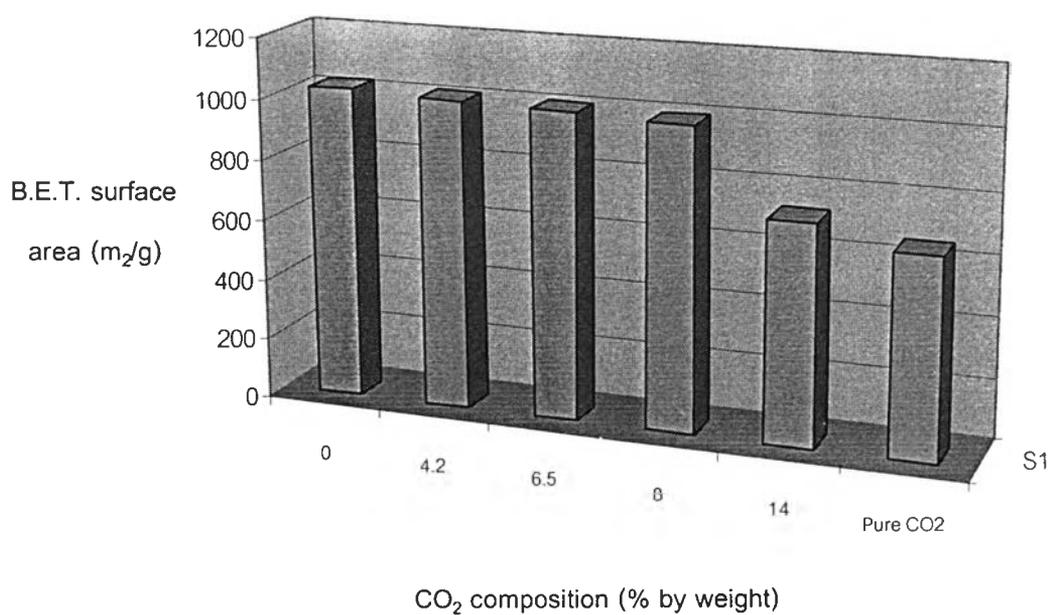
Figure 4.26 Effect of CO<sub>2</sub> (% weight) composition on B.E.T. surface area (950<sup>0</sup>C for 60 min, 0.60-1.18, 10g, air 0.005 l/min and superheated steam 10 g/min).
