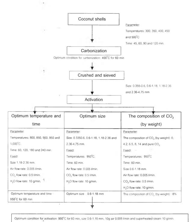
Figure 5.1 The optimum condition of the production of activated carbon from coconut shells by carbonized following by superheated steam and carbon dioxide
