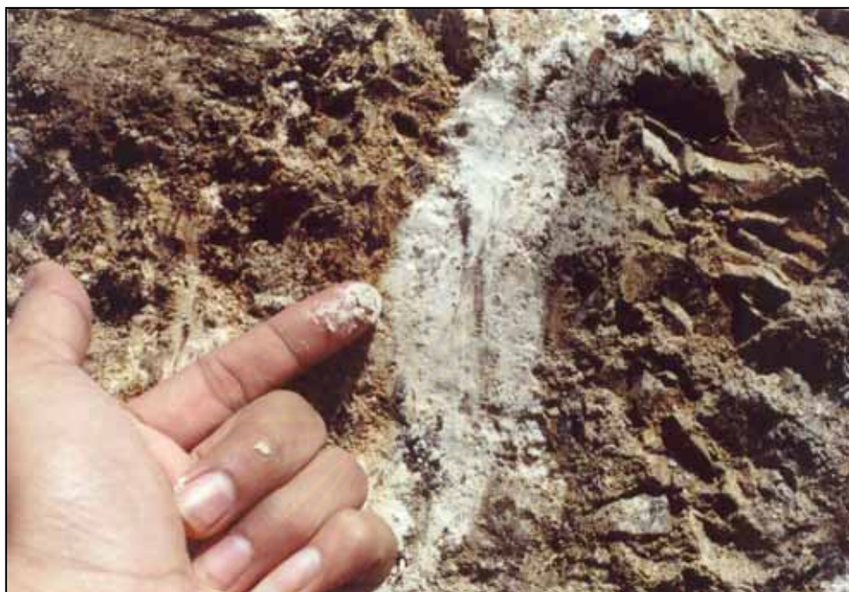
Figure 4.5 White veins of calcite cut into weathered Triassic mudstone bedrocks, west wall- side of the Ban Kaeng Kheap Trench.
