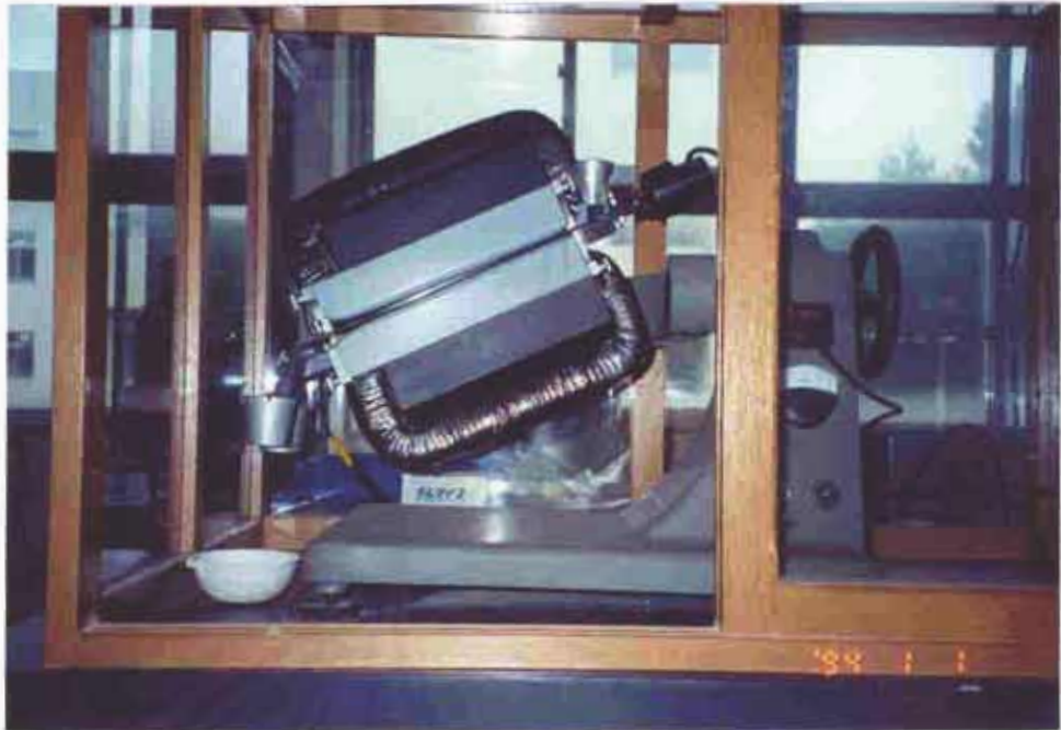
Figure 5.6 Frantz's isodynamic magnetrometer was applied to separate dark-colored minerals from light-colored less magnetic ones.
