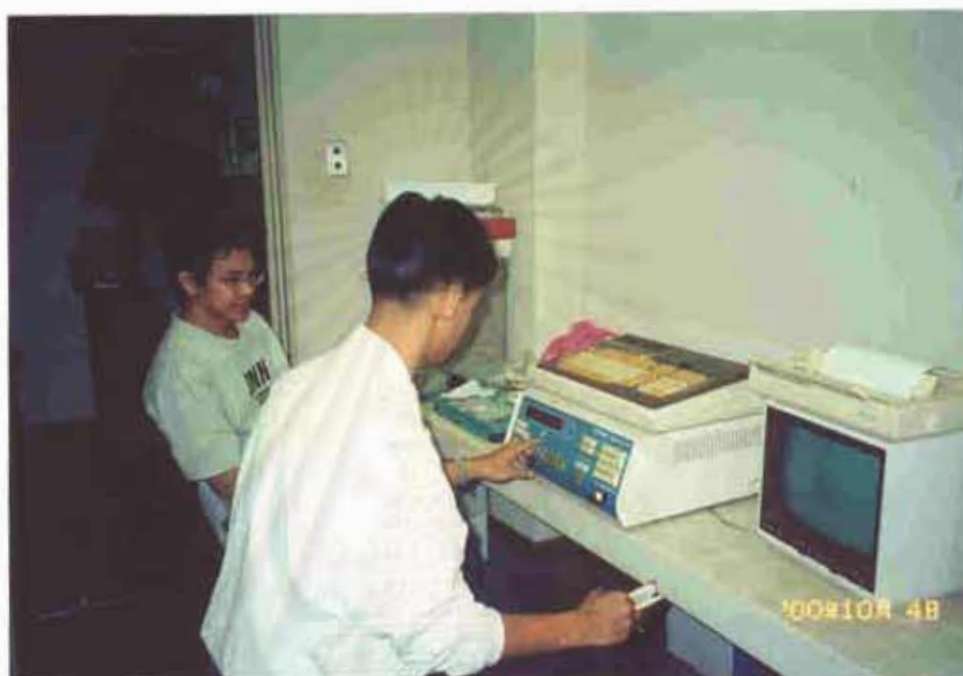
Figure 5.9 Common TL apparatus (the Kyokko 2500 TLD) with a photomultiplier (an instrument with Rutchut is left hand and the monitor (TV on the right) for showing TL signals
