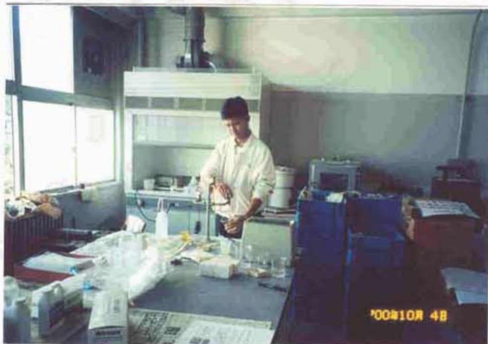
Figure 5.5 Samples are cleaned and washed with tapping water after etching with HF (Mr. Rutchut Nutthee is to scale)
