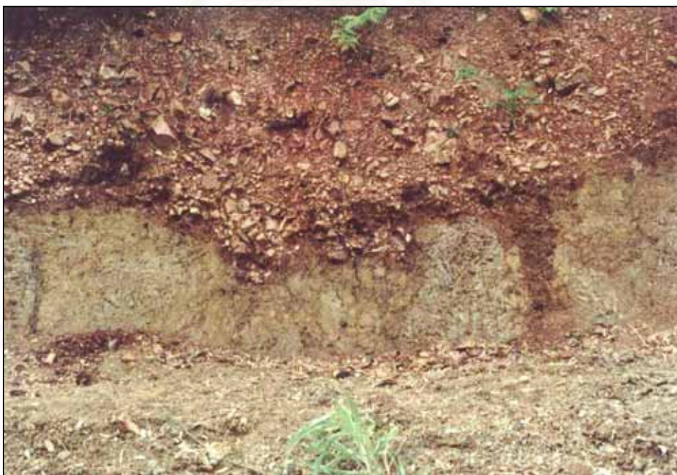
Figure 4.21 Close-up view of figure 4.17 showing well-defined colluvium wedge due to earthquake faulting.
