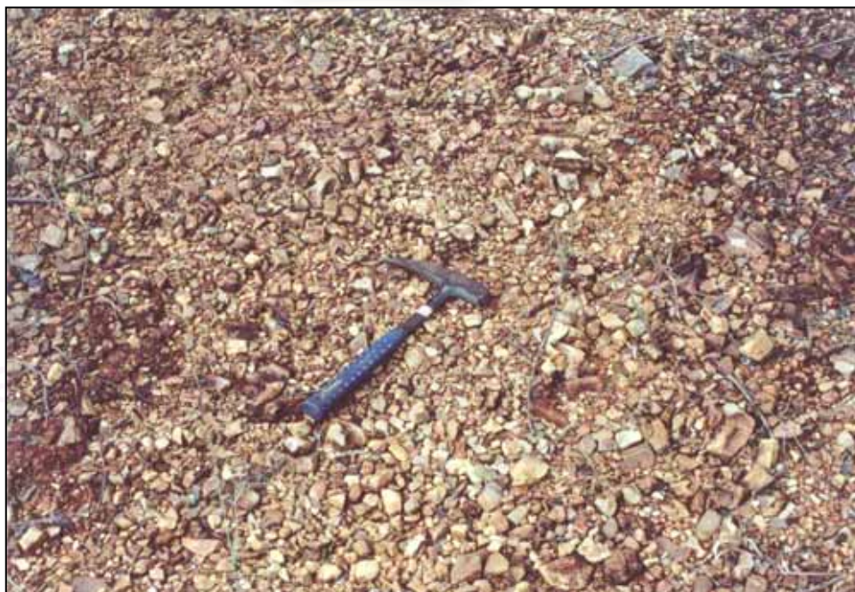
Figure 3.15 Close-up view (of Fig. 3.14) showing coarse fragments with high angularity of talus deposit.
