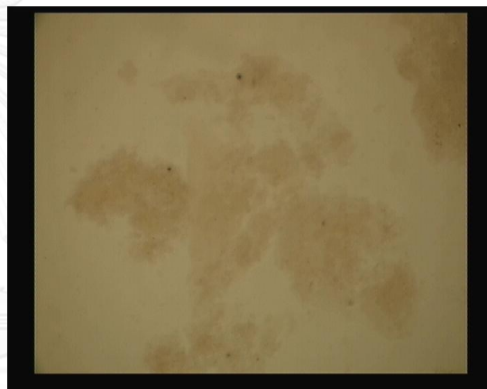
(b) Unmodified chitosan X10
