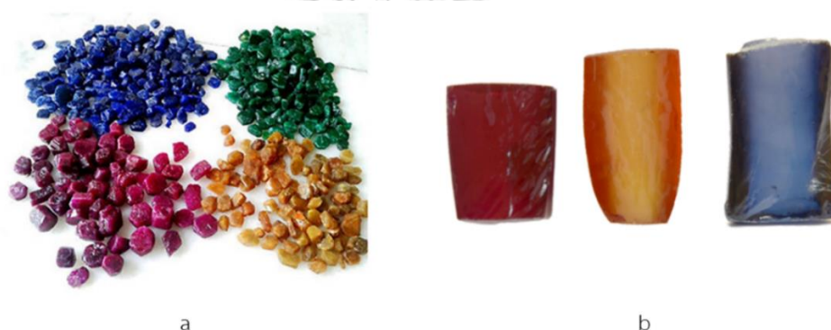
Figure 1 A comparison between of natural corundum (a) and synthetic corundum samples (b)
