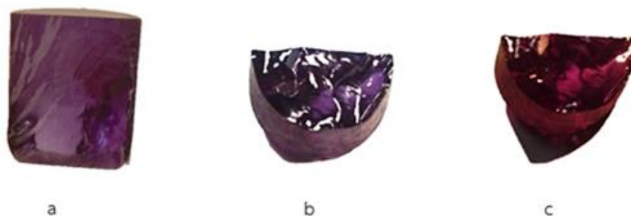
Figure 36 Color change apparent in the red synthetic corundum sample (R5): (a) side view in daylight, (b) top view showing bluish purple in daylight, and (c) top view showing purplish red in incandescent light.
