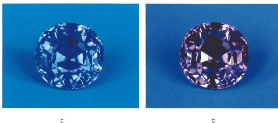
Figure 5 The color change in sapphire (a) Bluish color in daylight (b) Violetish red in incandescent light. (Gübelin et al., 1992).
