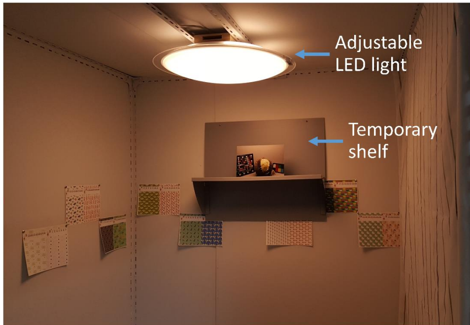
Figure 4- 6 Experimental room, temporary shelf fixed on the wall, and adjustable LED light mounted on the room ceiling.
