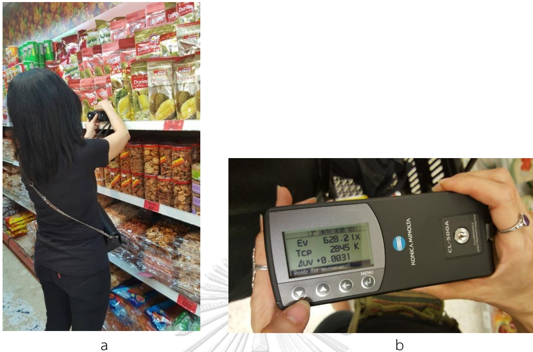
Figure 3- 6 Exploring CCTs and illuminances; a) At shelves selling package durian, b) CCT and illuminance were displayed.
