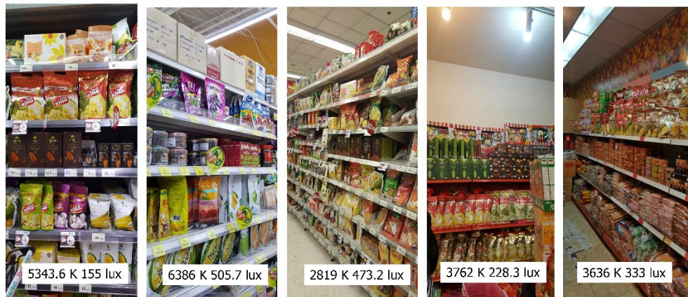
Figure 3- 7 The lighting conditions at shelves selling packed durian at 5 places of supermarkets and dried food stores.
