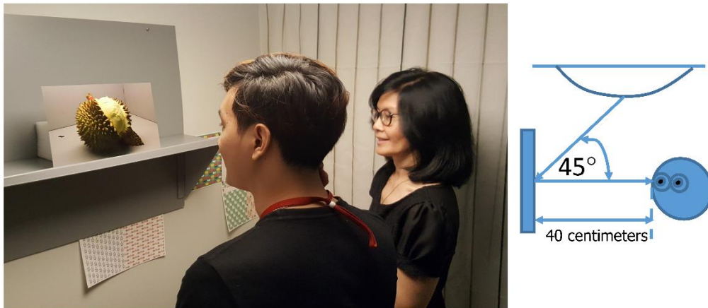
Figure 4- 9 Participant look at the durian image at the viewing of 45/0 degree in the distance of 40 centimeters.
