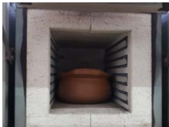
Figure.3.3 Muffled furnace (Carbolite ELF/11/14/201, England)
