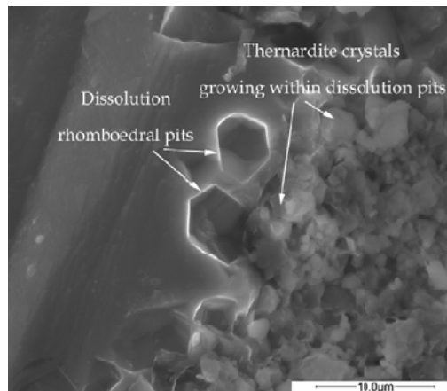
Figure 2.8 Scanning electron microscopy photomicrograph of calcite grains showing etch pits filled with \text{Na}_2\text{SO}_4 crystals (Ruiz - Agudo et al., 2007)
