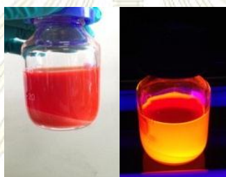
Figure 3.5 Physical appearance of the as-synthesized QDs under ambient light (left) and black light (right).
