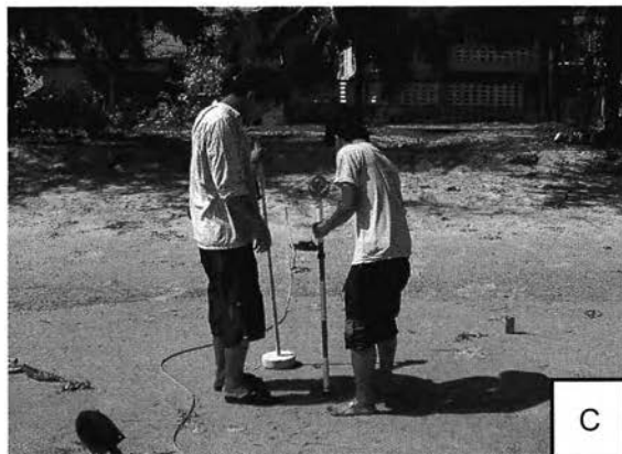
Figure 3.5 Photos showing the use of survey camera to measure shoreface position and slope. Picture A and B show how to set up survey camera and fix direction of shoreface profile. Picture C shows how to design and set up reference point, and the picture D shows the shoreface measure line perpendicular to the coastline.
