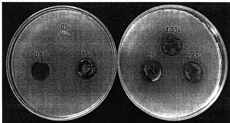
Figure 6.7 Illustration of the inhibition zone of the nAg-loaded SF films with containing in various \text{AgNO}_3 contents. The neat SF film was used as the control. The films were tested against with P. aeruginosa and incubated at 37^\circ\text{C} for 24 h.
