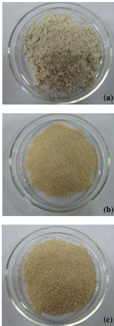
Figure 5.1 Tamarind kernel powder (a) small-size TKP (b) medium-size TKP and (c) large-size TKP
