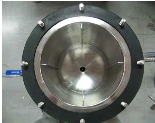
Figure B-3 Inner 10-liter closed mixing tank
