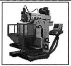
The FB-6 model is the continuation of the FB-4's global success story. The most important of the new features are hydraulic tool clamping and an external coolant system.
