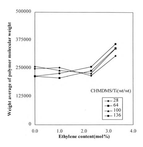
**Figure 4.10** Effect of CHMDMS concentration on weight average of polymer molecular weight.
