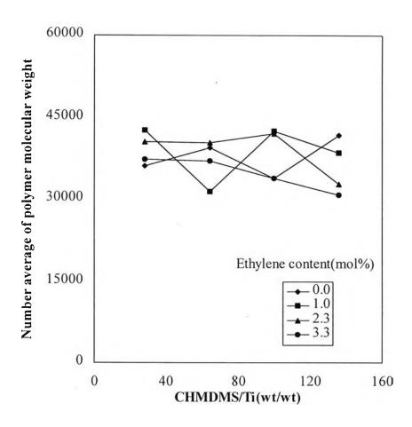
**Figure 4.5** Effect of ethylene content on number average of polymer molecular weight.
