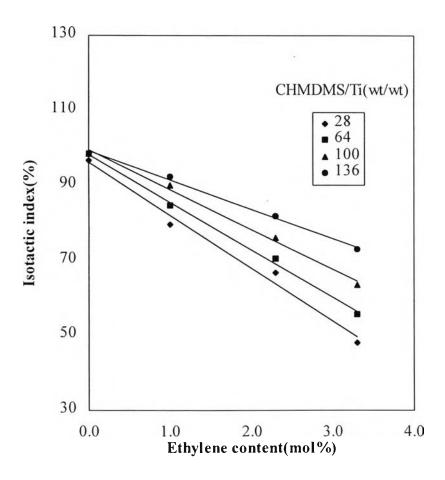
Figure 4.7 Effect of CHMDMS concentration on isotactic index.
