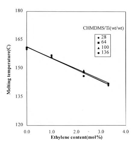
Figure 4.8 Effect of CHMDMS concentration on melting temperature.
