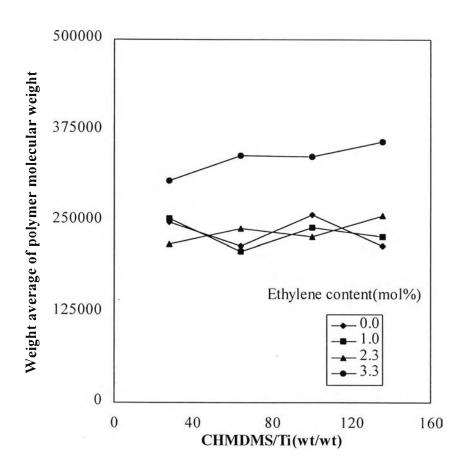
**Figure 4.4** Effect of ethylene content on weight average of polymer molecular weight.
