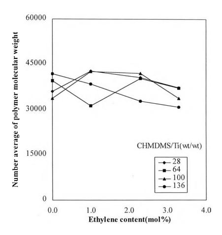
**Figure 4.11** Effect of CHMDMS concentration on number average of polymer molecular weight.
