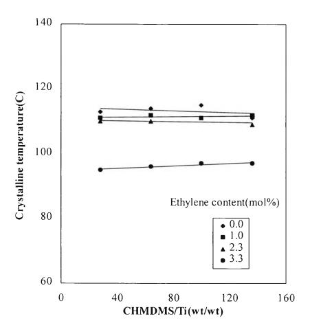
Figure 4.3 Effect of ethylene content on crystallization temperature.
