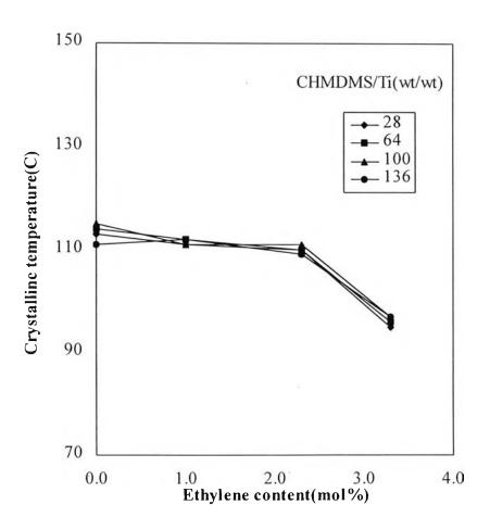
Figure 4.9 Effect of CHMDMS concentration on crystallization temperature.
