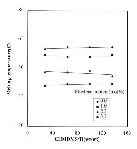
Figure 4.2 Effect of ethylene content on melting temperature.
