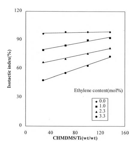
Figure 4.1 Effect of ethylene content on isotactic index.
