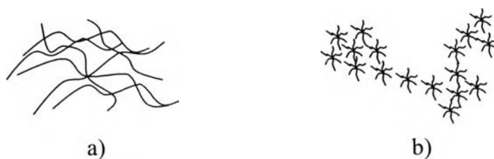
Figure 2.1 Schematic representation of microstructures upon gel desiccation: a) acid-catalyzed b) base-catalyzed.
