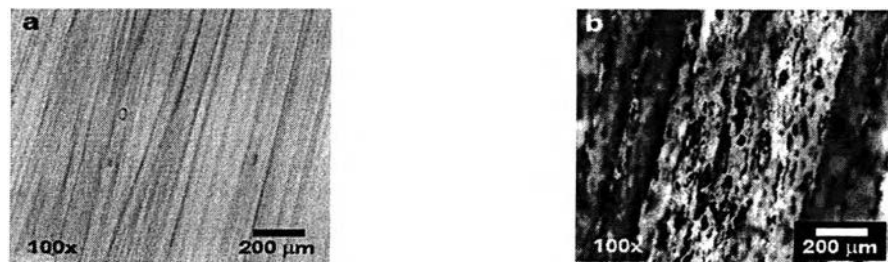
Figure 6.6 Representative microscopic images of (a) calcium alginate and (b) 10% w/w chitosan-spotted alginate yarns after immersion in 0.01% w/v Amido Black 10B aqueous solution for 8 h.
