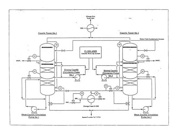
Figure 1.1: Caustic tower diagram
