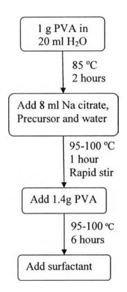
Figure 3.1 Flow chart shows the electrospinning solution preparation.
