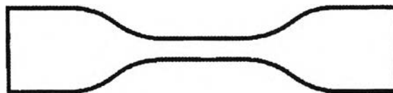
Figure 2.5 Dumbbell shaped test piece for tensile testing.
