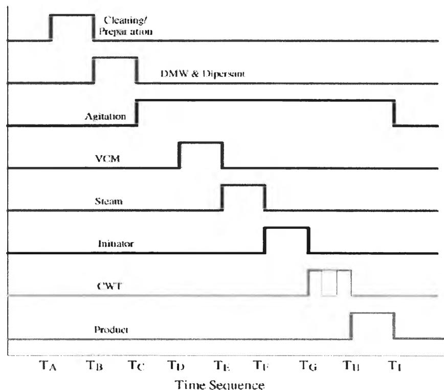
**Figure 2.10** Switching signal mode for PVC batch process (Rizal, Tani, Nishiyama and Suzuki, 2006)
