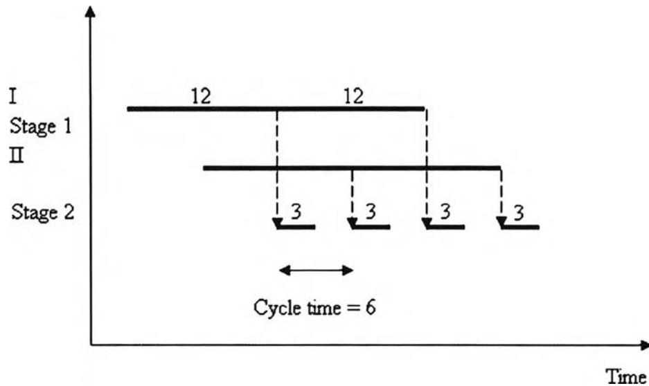
Figure 2.6 Plant with parallel units in fermenter (Biegler, 1999)
