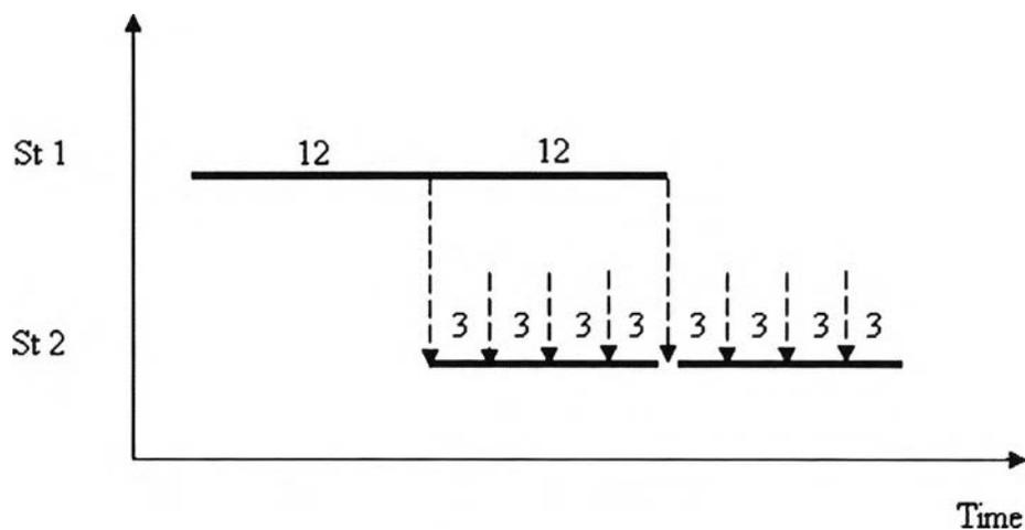
Figure 2.7 Fermentation plant with intermediate storage (Biegler, 1999)
