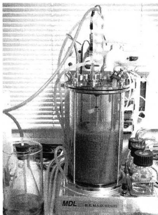
Figure 17 Ethanol fermentation by separate hydrolysis and fermentation method in 5L fermentor (B.E. Marubishi, model 10L, Japan).
